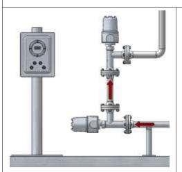
The horizontal installations are acceptable if the flow speed is higher than 2 feet per second.
