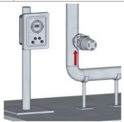
Mounted on a vertical line at 90°
